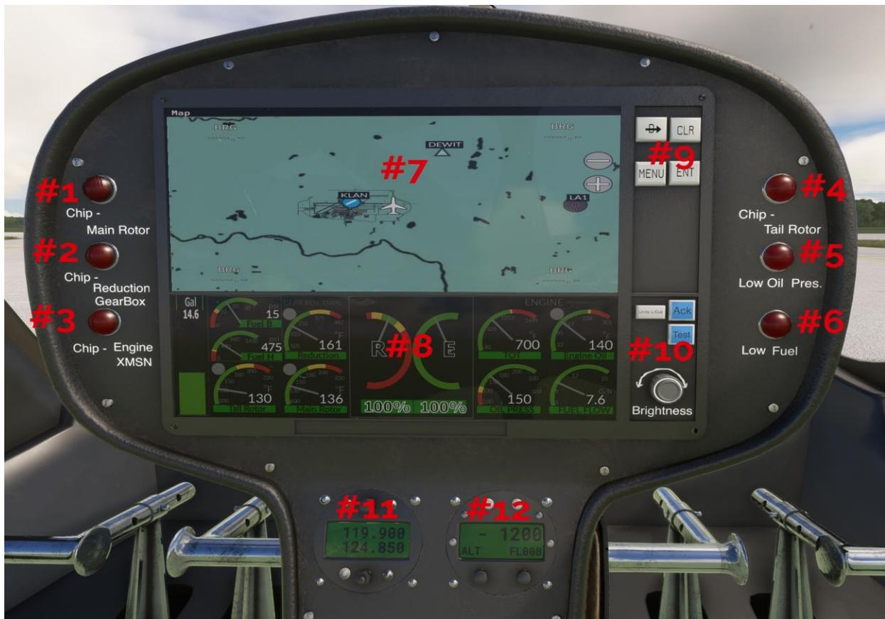
1. Chip Detector Main Rotor Gearbox
