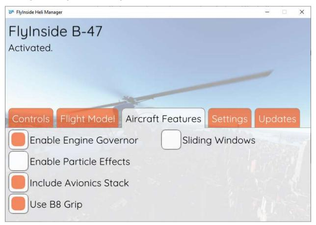
"Enable Engine Governor" allows you to switch the included engine governor on and off. When on, the helicopter automatically maintains 100% rotor RPM if able. If turned off, you'll need to manually control the RPM via throttle, as described at the end of Chapter 3.
